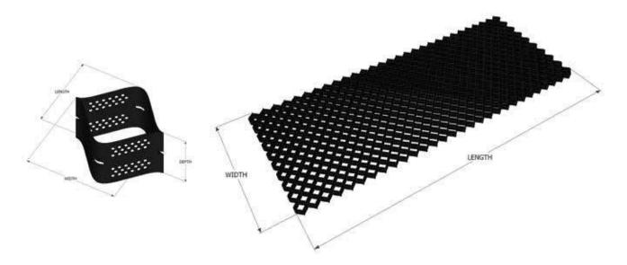
StrataWeb® utilizes interconnected strips of polymer, meticulously welded together at intervals to form a robust and flexible mattress. Filled with granular material, the resulting cellular confinement system efficiently transfers compressive and tensile stresses from heavy loads, providing higher load support capacity than any other geosythetic product available.
