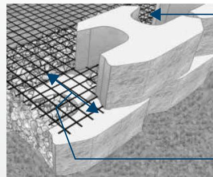
Staggered hollows filled with gravel become integral part of fascia, contributing support and stability to the fascia
