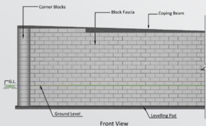
Schematic diagram of RS Wall with precast concrete StrataBlock™ fascia
