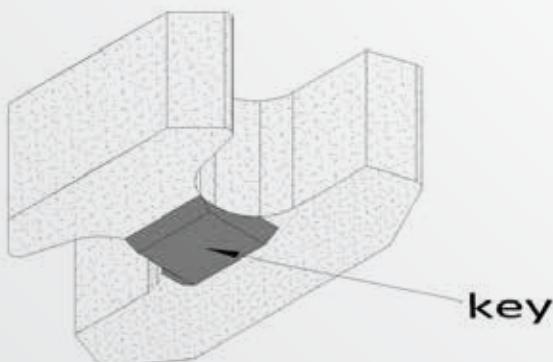
16mm shear key for StrataGrid™ connection
