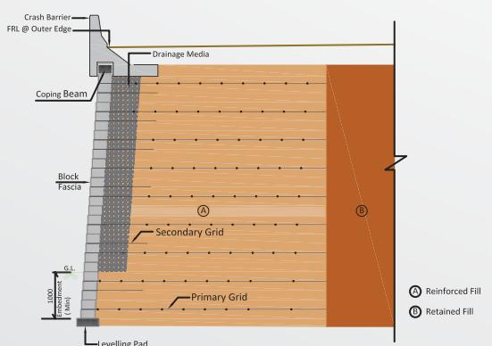
Schematic diagram of typical cross section of reinforcement soil (RS) wall
